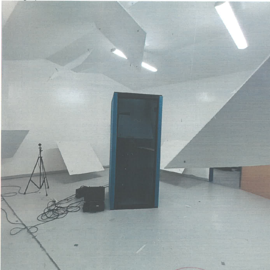
Fig. 1 sample installed in the reverberation chamber
